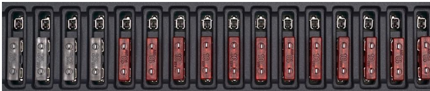
Figure 14. Fuses In Normal Operation
